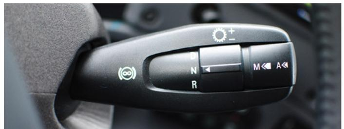
The shift lever includes gear, auto/manual mode and engine brake selection for excellent ergonomics.
